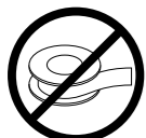
Pipe tape is not recommended.
