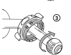
3. Thread pivot ball onto shower pipe and hand-tighten to a snug fit.
