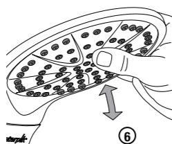
6. To adjust the angle of the drencher, simply pull the head up or down to desired position. The head will click into place.
