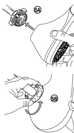
5. Hold threaded collar of shower head up to pivot ball (5A), adjust shower head to desired position and tighten nut in clockwise direction until secure. (5B)
