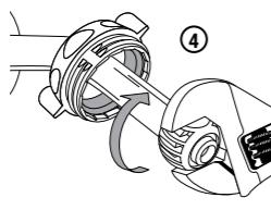
4. With an adjustable wrench or pliers, tighten pivot ball an additional 1/4 to 1/2 turn. Wrap pivot ball with a cloth if you are using pliers.
