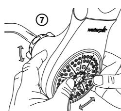
7. To adjust the fixed mount spray direction, hold fixed mount with both hands and rotate fixed mount up or down on pivot ball.
