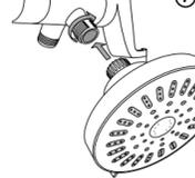
7. Attach fixed mount shower head by threading pivot ball onto diverter. Tighten securely with wrench. Wrap pivot ball nut with a cloth if you are using pliers. **Do not over tighten.**
