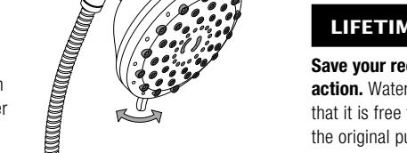
**Note:** When adjusting mode patterns make sure that only the face of the fixed mount shower head rotates or you may loosen shower head from diverter.
